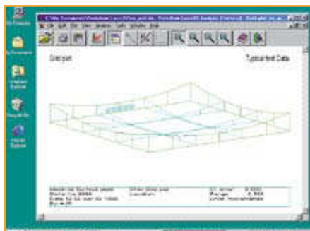
These are the typical plots obtained from a flatness measurement. The top graph shows a Moody plot type whilst the bottom shows a typical Grid plot type.
