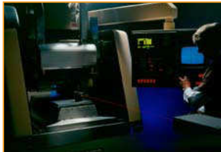
Wafer dicing machine calibration (photograph courtesy of Manufacturing Technology Inc)
