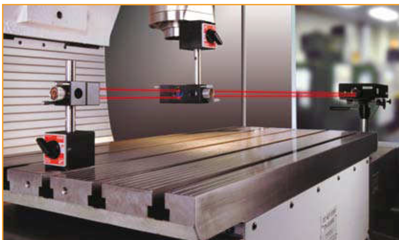
X axis linear positioning measurement on a VMC
